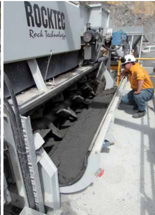
The pugmill with the cover open, showing the mixing paddles.
